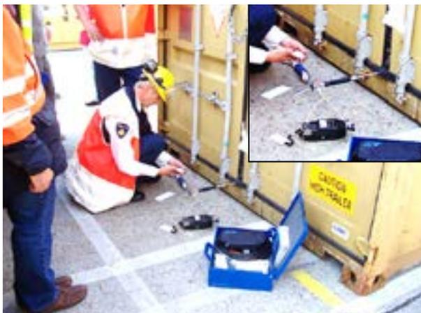
Testing for toxic gas using a "photo ionization gas detector prior to opening shipping container. (Courtesy of the Netherlands - ILT)
