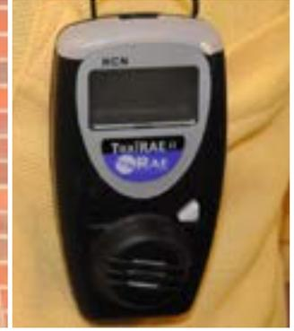
Gas specific pocket monitors may be worn to provide warning against elevated H<sub>2</sub>S (or other gases) to provide audible warnings when thresholds are exceeded. (Courtesy of United States - EPA, Canada - DOE)
