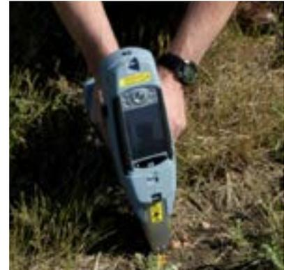
Spot sampling with handheld X-ray fluorescence analysers can help quickly map out metal contaminated zones.
