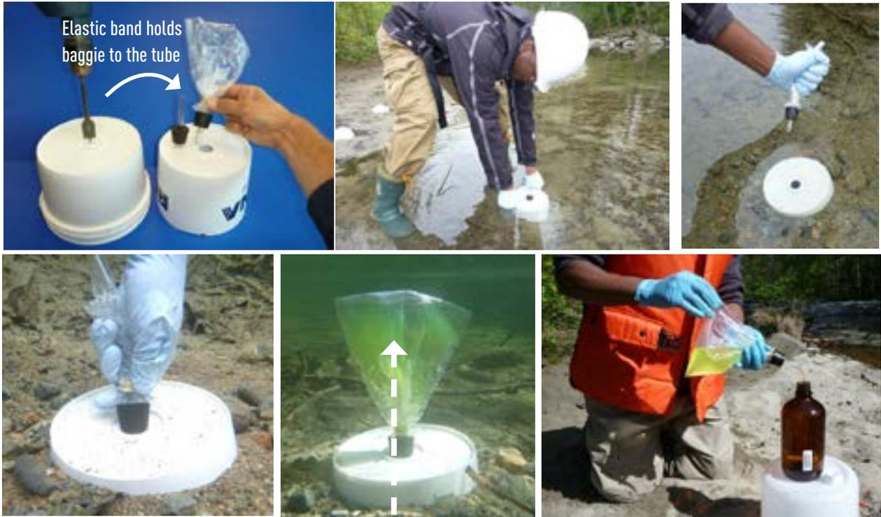
**Option 2** Sampling using shallow piezometers
