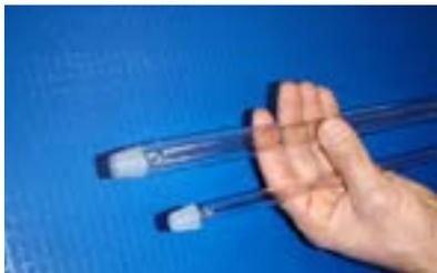
Fritted glass "Barrel Thief" can collect a composite sample from a barrel which may contain layers of different liquid wastes.
