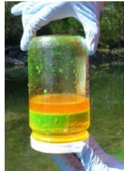
Drum liquid sample is dispensed into a glass sample jar for organics analysis. A duplicate can be placed in a clear glass jar to illustrate multiple layers of chemicals. Hazardous liquid waste of higher density (usually chlorinated organics) may be hidden under a benign layer (commonly called cocktailing).
