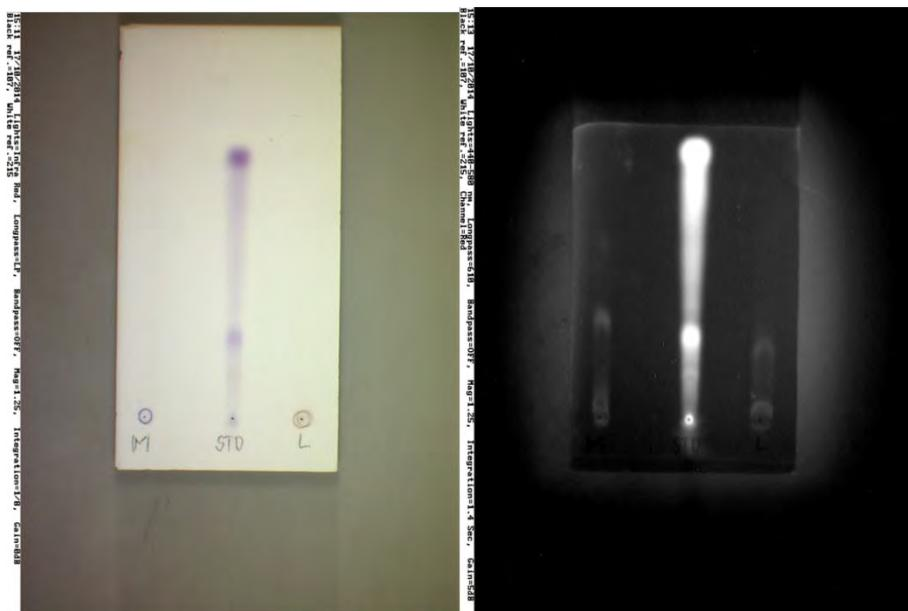
Figure D2. Writing instruments M and L separated via TLC: (left) separation visualized in ambient conditions, (right) TLC plate visualized in VSC under spot light (440-580nm) exhibiting luminescent spots that are invisible to the naked eye (colorless).
