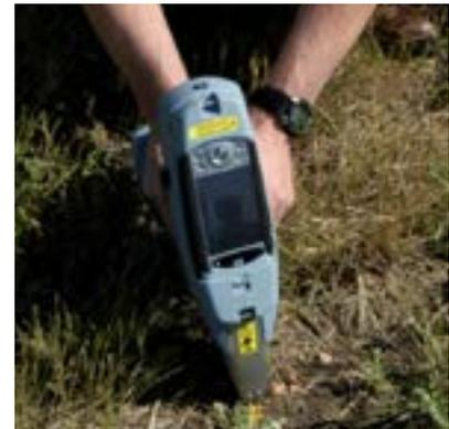
Spot sampling with handheld X-ray fluorescence analysers can help quickly map out metal contaminated zones. (Courtesy of United States - EPA)
