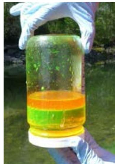
Drum liquid sample is dispensed into a glass sample jar for organics analysis. A duplicate can be placed in a clear glass jar to illustrate multiple layers of chemicals. Hazardous liquid waste of higher density (usually chlorinated organics) may be hidden under a benign layer (commonly called cocktailing).
