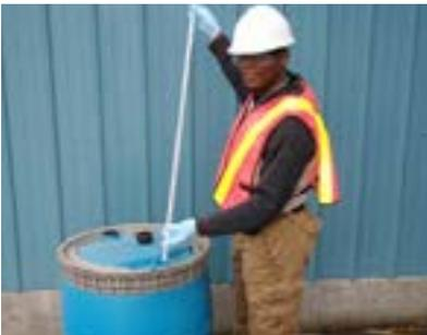
Sampler should wear appropriate safety equipment such as hard hat, respirator, safety glasses, gloves and chemical resistant suit.
