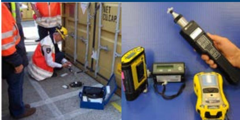
Before a suspected hazardous waste shipping container is opened it should be tested with a gas sniffer.
