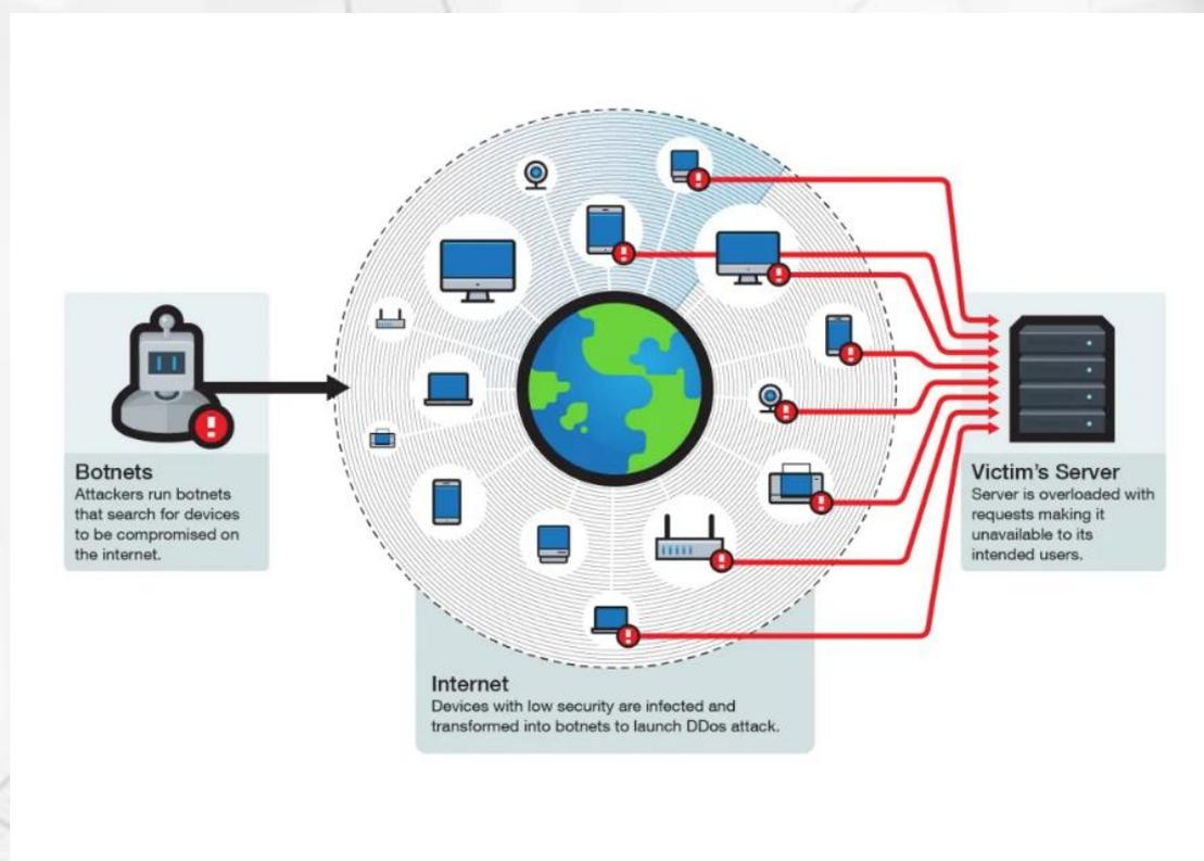
Figure 4: How a Botnet works, Trend Micro
