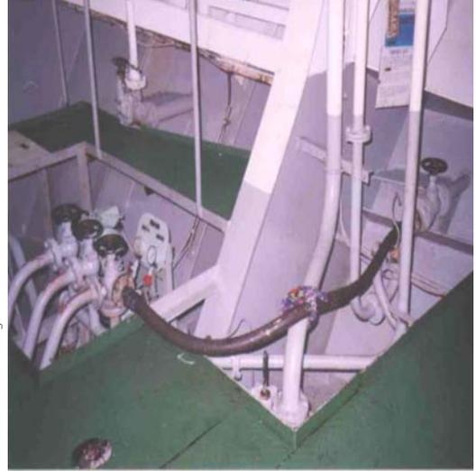
18. Bypass hose connected from the bilge manifold directly to the Overboard Discharge Valve.
