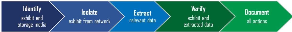
Figure 7. Data Extraction Process on Mobile Devices
