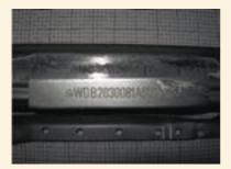
Make sure the stamped chassis number corresponds with the vehicle identification number which is mentioned on the car documents as well as on small plates elsewhere in the vehicle.
