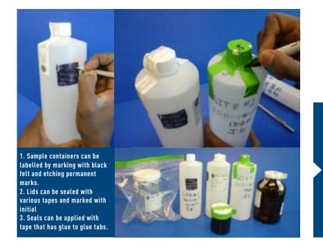
FIGURE 2.10: Examples of various numbered labels and etching tools. (Courtesy of Canada DOE)
