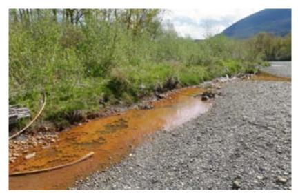
4. Test the shallow water near the bottom sediments (epibenthic zone) for pH, dissolved oxygen, temperature and conductivity. Extreme pH ranges, high temperature, low dissolved oxygen and high conductivity may indicate contamination
