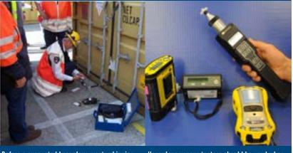
Before a suspected hazardous waste shipping container is opened it should be tested with a gas sniffer.
