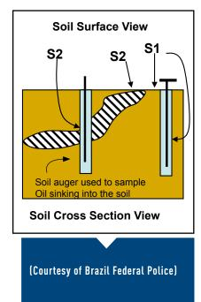
Use a clean stainless steel scoop and soil auger at each site to collect samples.
