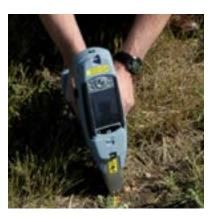
Spot sampling with handheld X-ray fluorescence analysers can help quickly map out metal contaminated zones. (Courtesy of United States - EPA)
