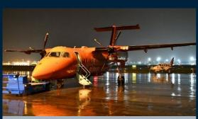
Transport **Canada** deployed its National Aerial Surveillance Program conducting 20 night flights to detect pollution incidents. Aircrafts are equipped with night vision cameras, Side Looking Airborne Radar (SLAR), Electro-optical Infrared Cameras (EO/IR) and Infrared/Ultraviolet Line Scanners (IR/UV).
