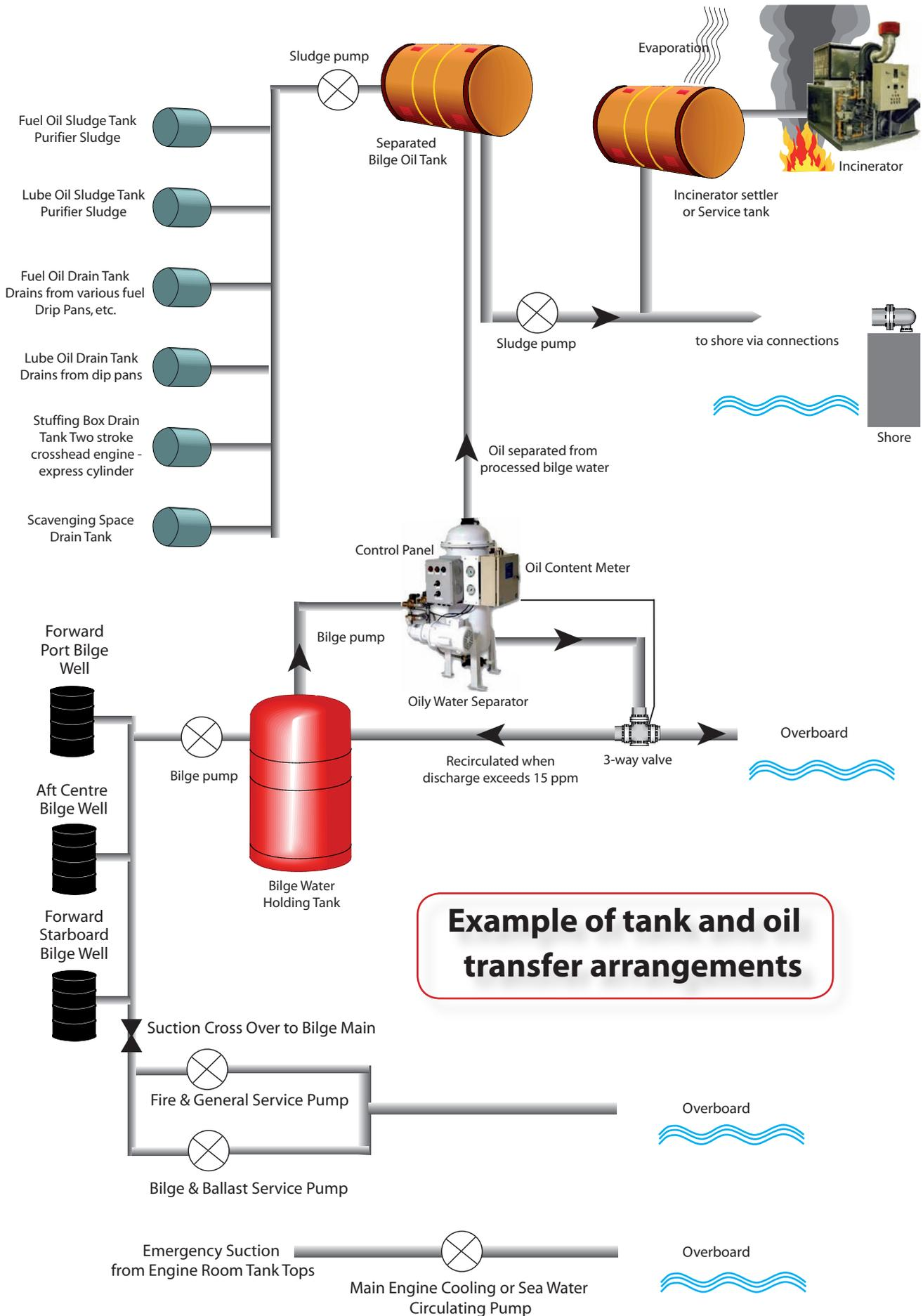
**Example of tank and oil transfer arrangements**
