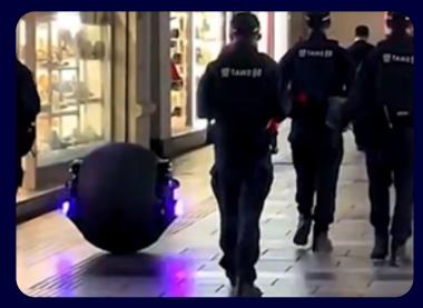
Its advanced sensors enable it to detect abnormalities and unusual events within its surroundings, while its facial recognition software allows the robot to identify known criminals for enhanced security. When the RT-G detects a threat or a known criminal, it can either call for backup from other robots in the area or law enforcement officers.
