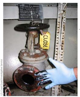
10. Oily residue found inside Overboard Discharge Valves.
