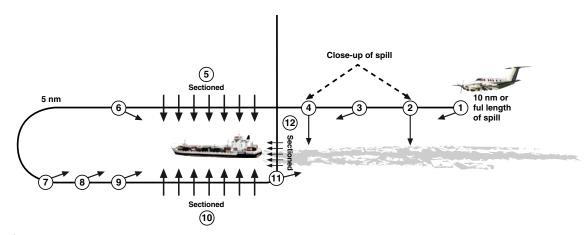
25. Example of flight plan for vessel trailing discharge and suggested photograph positions.
