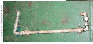
14. Fabricated piping used to bypass Oily Water Separator.
