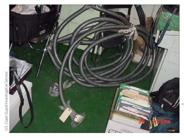
12. 40-foot flexible bypass hose with oil residue.
