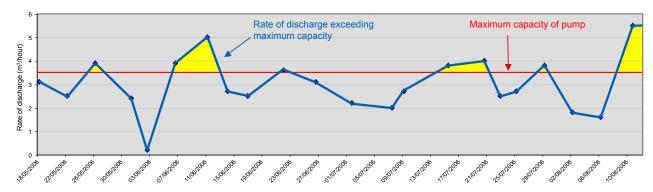
6. The table shows records of discharges in excess of the maximum capacity of the OWS which is 3.5 cubic meters. Such discharges are made discreetly.
