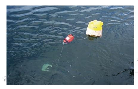
28. Sampling buoy that can be released from an aerial surveillance plane, developed in cooperation with Swedish Coast Guard.
