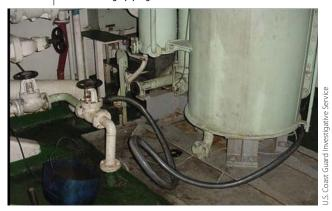
16. Bypass hose connecting bilge piping to Marine Sanitation Device discharge piping.
