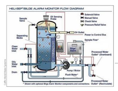
3. Example of Oily Water Separator with bilge alarme.
