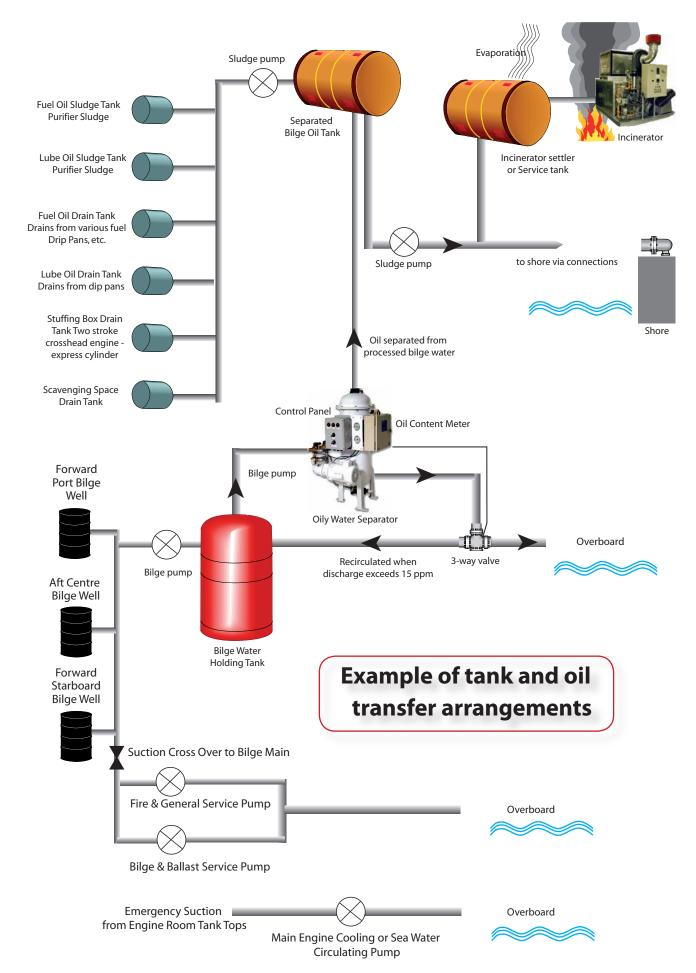
Separator (OWS). This equipment is required to be designed and tested to separate oily water mixtures to a maximum limit of 15 parts oil to one million parts water (15 ppm). The equipment may be fitted with an Oil Content Meter (OCM) and automatic stopping device which prevents the discharge of any effluent above the 15 ppm limit, but this is only required on vessels over 10,000 gt.
