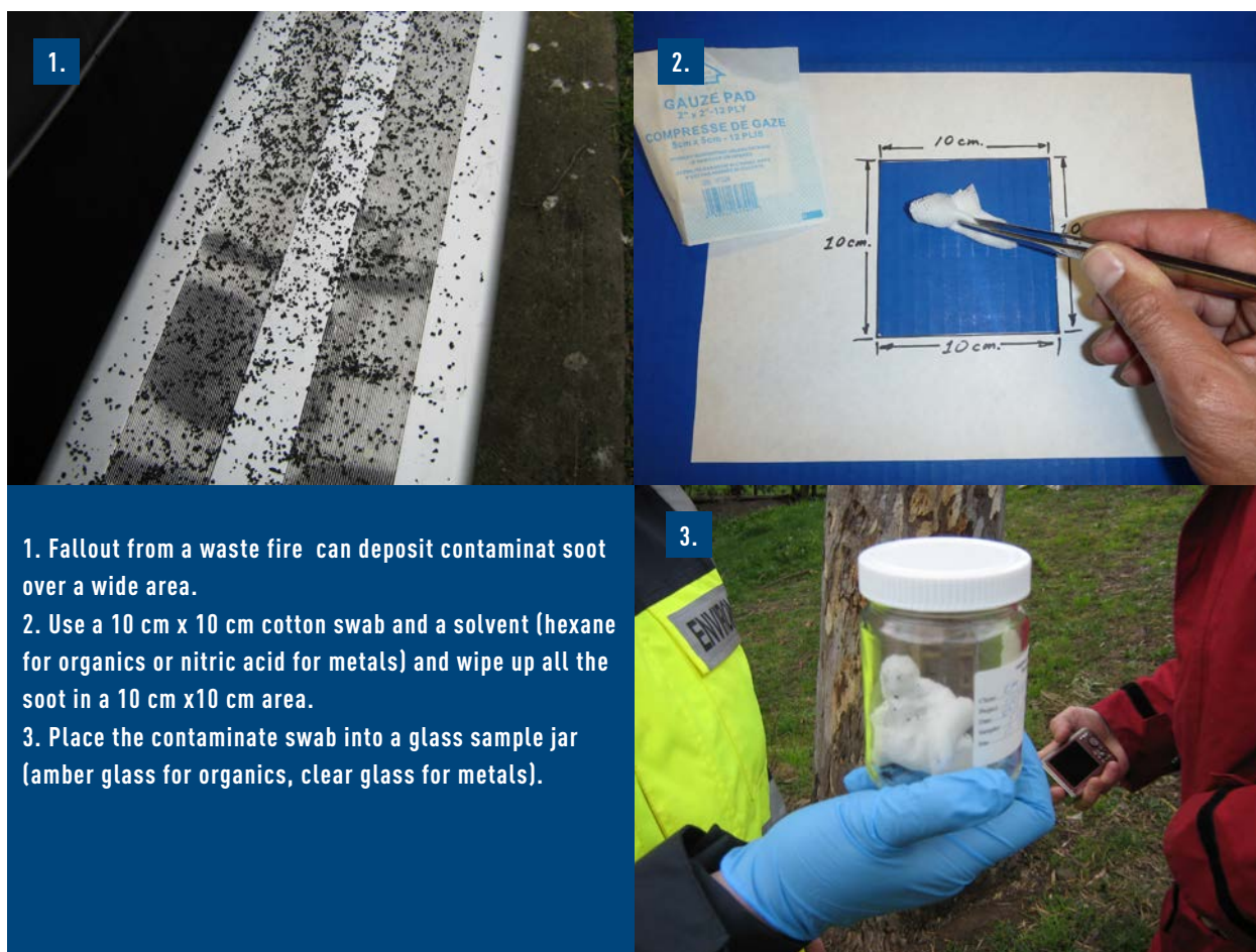
FIGURE 7.1: Swab/wipe sample of fallout, with 100 cm 2 template and solvent and tweezers. (Courtesy of Genesis Environmental Sciences Ltd.)
