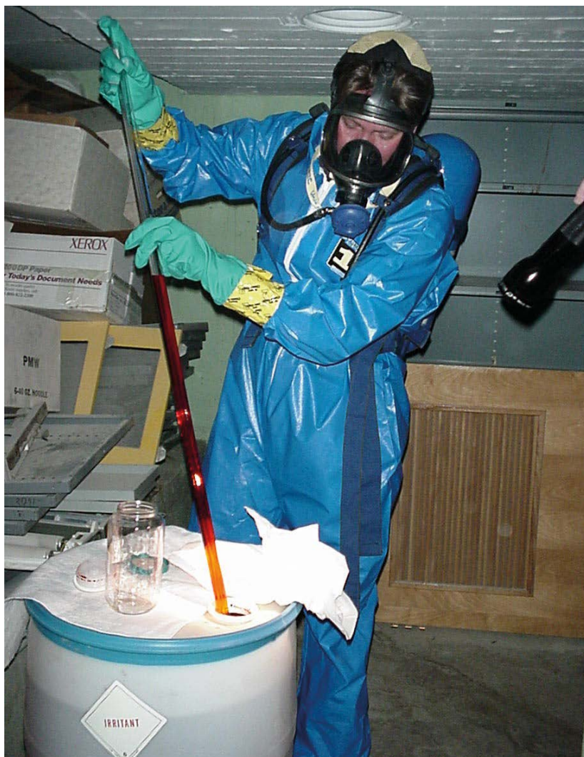
FIGURE 4.2: Glass composite liquid waste sampler “COLIWASA” or tube sampler. External glass tube contains the sample and the internal glass tube has a stopper which prevents sample from leaking out. (Courtesy of United States - EPA)
