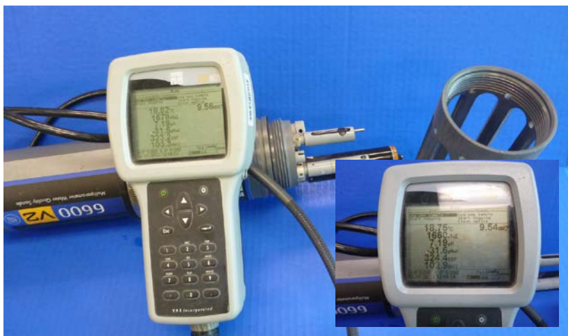
FIGURE 3.1: Single and multiparameter meters can monitor pH, dissolved oxygen, conductivity, salinity, temperature and other criteria depending on the number and types of probes. (Courtesy of Canada – DOE)
