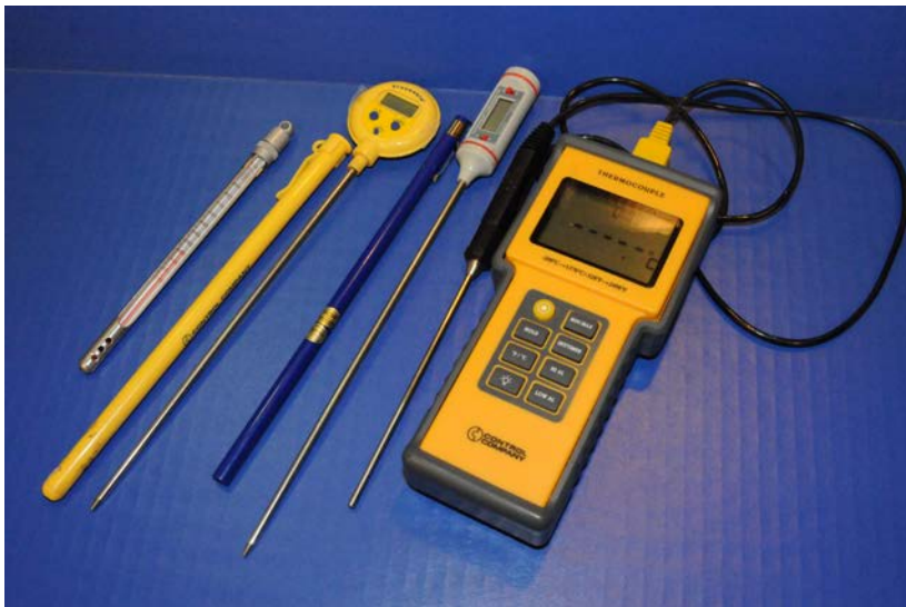
FIGURE 3.3: Temperature probes range from glass thermometers in a stainless steel casing to single measure or multiple measure probes which can record data. (Courtesy of United States and EPA/Canada - DOE)
