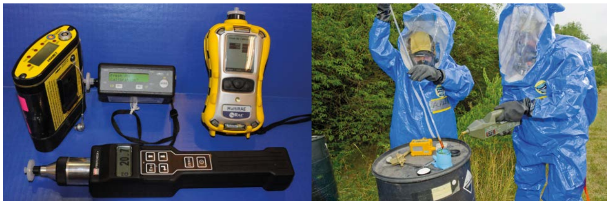
FIGURE 8.3: Portable photo ionization detectors. (Courtesy of United States - EPA, Canada - DOE)
