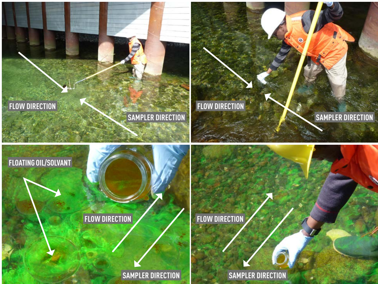
FIGURE 6.1: Surface water grab sample being collected using a hand method and facing upstream, a telescoping pole from shore, bridge or boat. (Courtesy of Canada – DOE)
