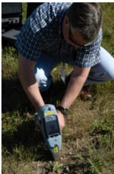
FIGURE 3.8: Hand-held X-ray fluorescent (XRF) analysers have the capability to quantify or qualify nearly any element from magnesium to uranium, depending on specific instrument configurations. These are particularly useful for heavy metals contaminated sites. (Courtesy of United States - EPA)
