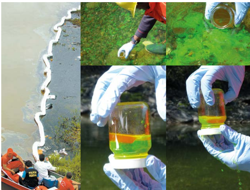
FIGURE 6.5: Collecting samples of floating liquids and petroleum products. (Courtesy of Brazil – Federal Police and Canada - DOE)
