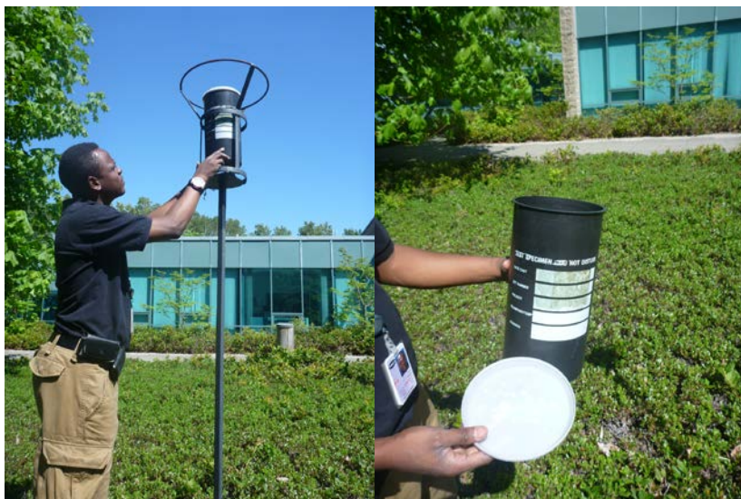
FIGURE 8.2: Dustfall sampler lid is removed and positioned in the sampler. (Courtesy of Canada - DOE)
