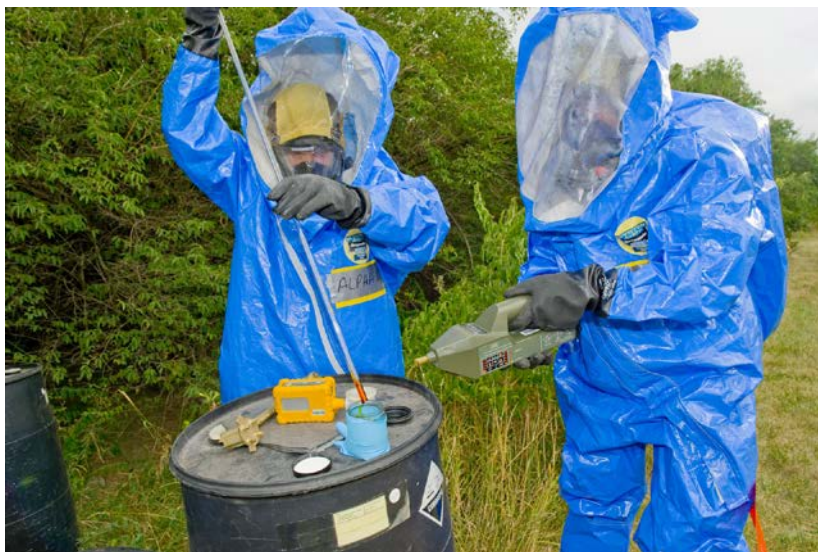
FIGURE 6.6: Using a gas vapour analyser and a glass COLIWASA sampler to collect a sample of unknown substance from a barrel. (Courtesy of United States – EPA)
