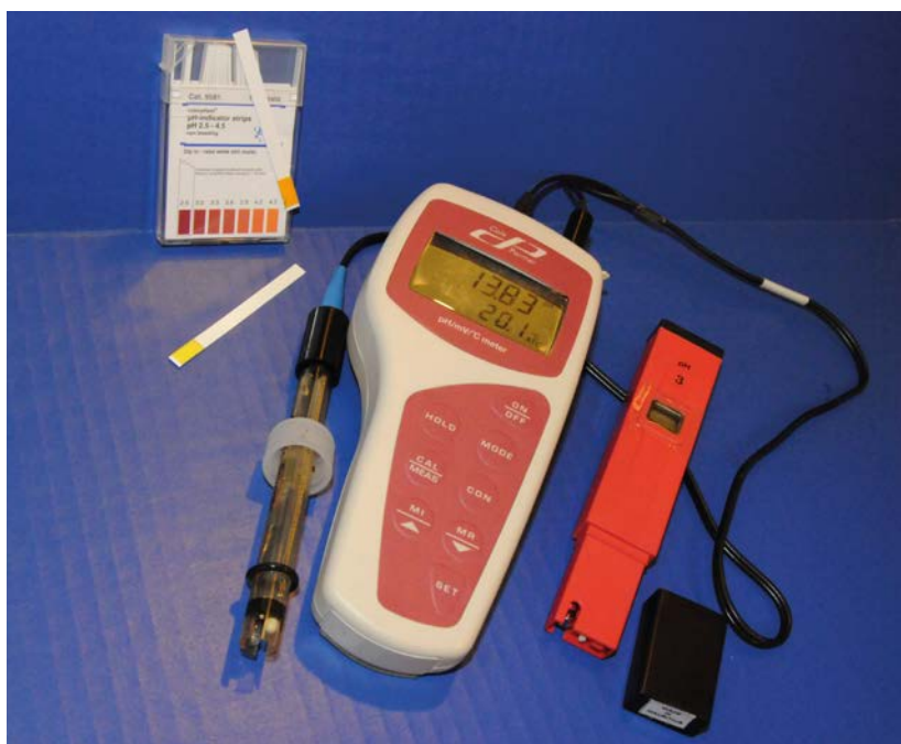
FIGURE 3.2: Single use pH paper or single parameter pH meters. (Courtesy of United States - EPA/Canada - DOE)
