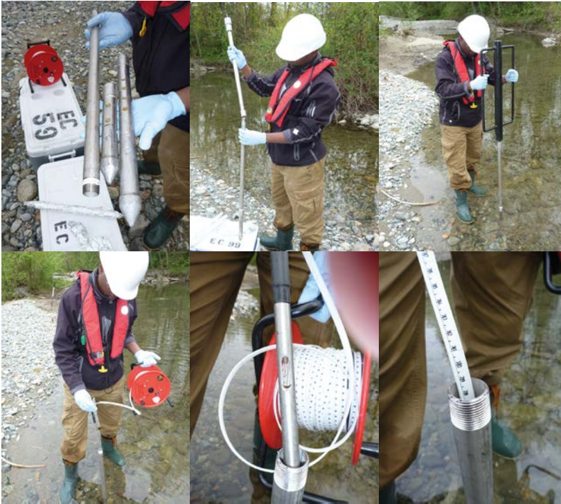
FIGURE 6.13: Installation of shallow piezometers using a slide hammer, and measurement of groundwater elevation. (Courtesy of Canada – DOE)
