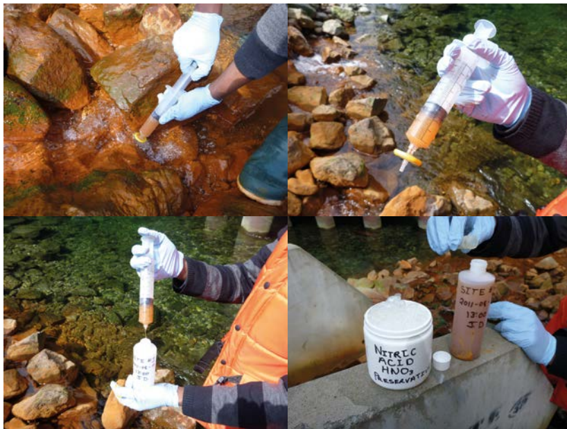
FIGURE 6.16: Syringe and 0.45 micron Filter to collect dissolved metals water sample. (Courtesy of Canada - DOE)
