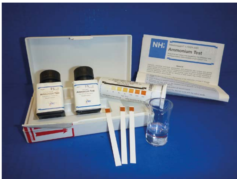
FIGURE 3.4: Portable ammonia test kits are valuable for field measurements as ammonia is volatile and should be measured as soon as possible. (Courtesy of Canada – DOE)
