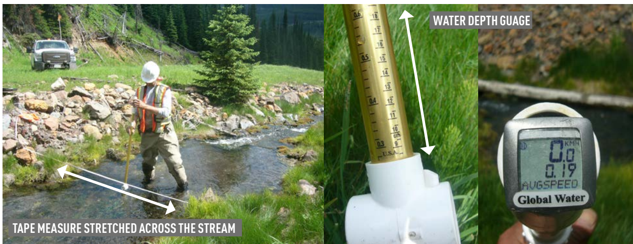
FIGURE 5.3: Use of tape measure and portable flow meter to estimate stream flow. (Courtesy of Canada – DOE)
