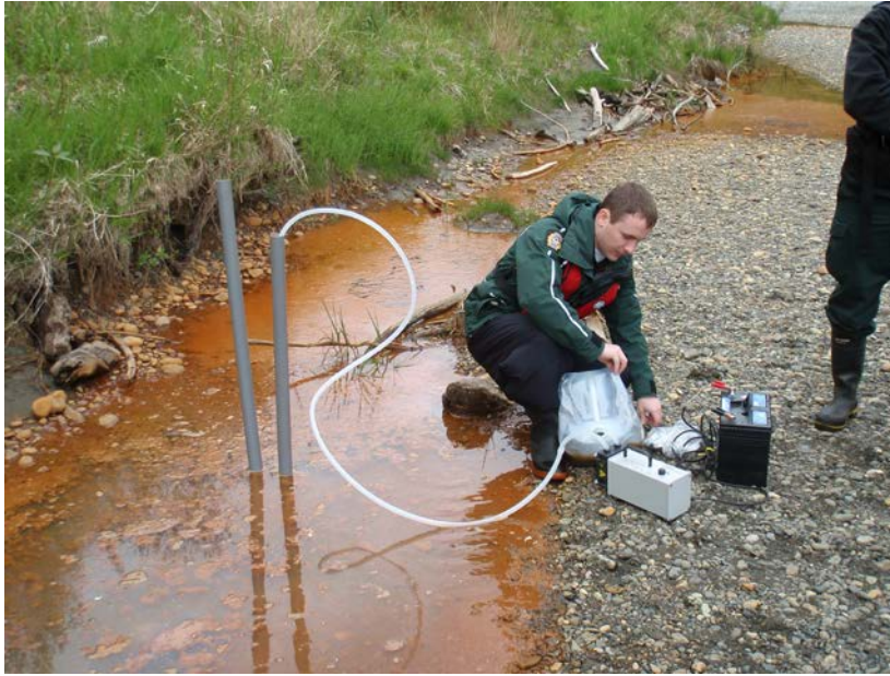
FIGURE 6.14: Grab sample being collected from a shallow piezometer using a peristaltic pump. (Courtesy of Canada - DOE)
