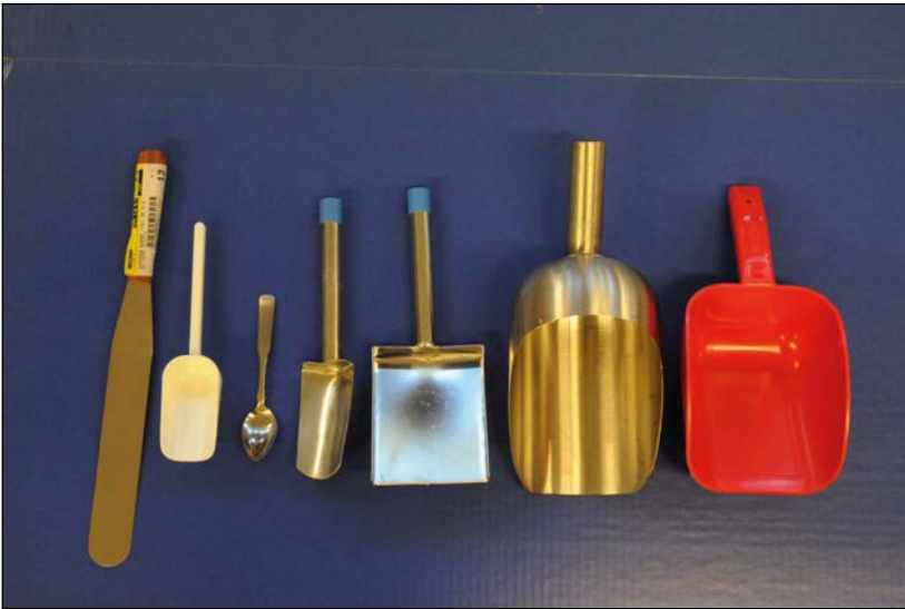
FIGURE 4.10: Typical reusable stainless steel and disposable plastic sample scoops (Courtesy of United States - EPA/Canada - DOE)
