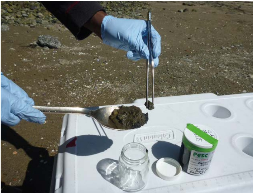
FIGURE 7.2: When collecting a sediment sample attempt to collect uniform fine grained material. Remove large rocks or woody debris which cannot be digested. (Courtesy of Canada – DOE)
