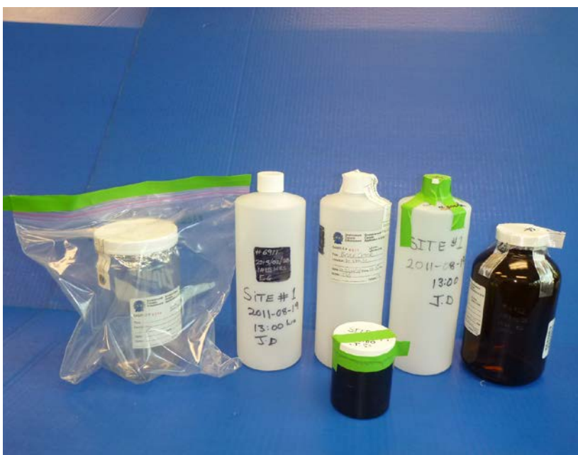
FIGURE 11.1: Legal seals can be made of prepared tamper-proof tape or of common tape. It is important to initial the seams of the tape and keep markings to a minimum to uniquely identify the sample. (Courtesy of Canada - DOE)
