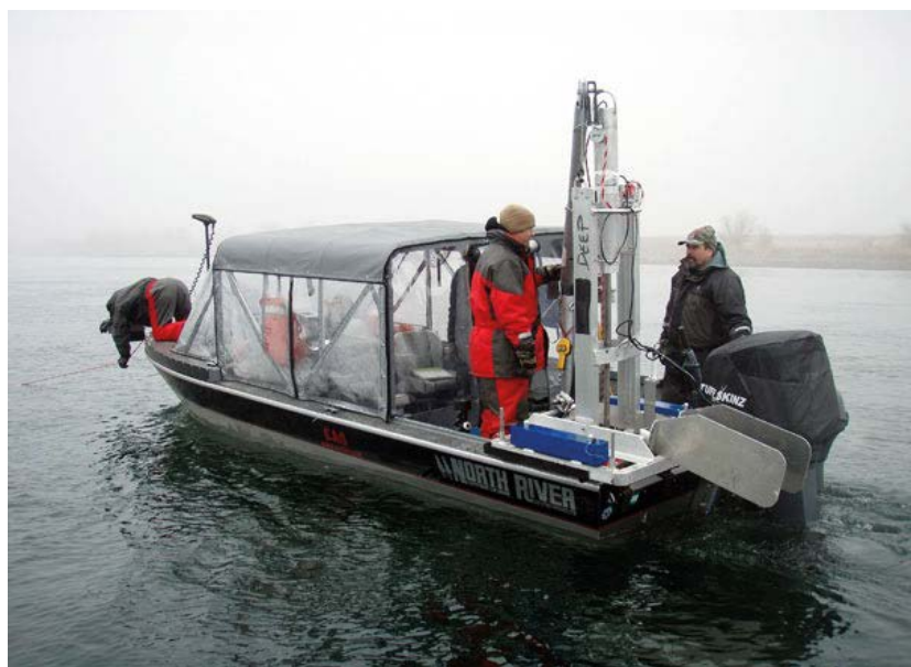
FIGURE 4.7: Neptune hyporheic water sampler. (Courtesy of Coastal Monitoring Associates – USA)
