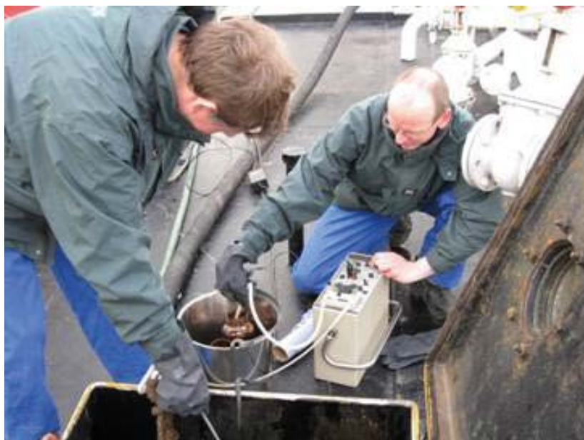
FIGURE 6.7: Sample collected from a bulk tank using a peristaltic pump. Note : if hazardous vapours are present, respirators would be required. (Courtesy of the Netherlands - NFI)
