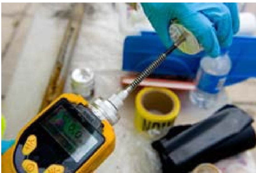
FIGURE 7.5: Using a photo-ionization detector, insert the detector nozzle through the aluminum foil and take a head space sample to determine if there are hydrocarbon or organic fumes. (Courtesy of United States - EPA)
